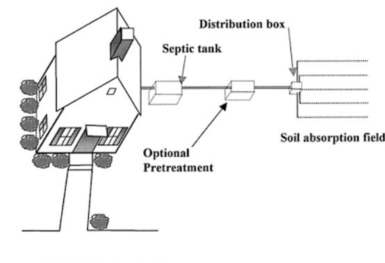
**Figure 1.** Schematic of on-site waste disposal system.
